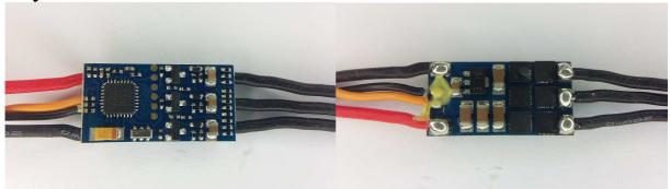
The ESC supports 2S to 4S operation. It supports damped light mode. It supports overtemp protection and bootloader on input plug (ICP1). Since it uses ICP1 as input, it runs smooth also with OneShot125 input signal. Switching speed is quite fast, although high side is slow to turn on. Both high side and low side are Nfets. It uses the "DYS SN20A .." code.
