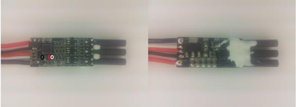
The ESC supports 2S to 4S operation. Switching speed is not fast, high side is slow to turn on. Low side is Nfets and high side is Pfets.
