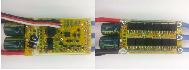
The ESC supports 2S to 4S operation. Switching speed is slow. Fet resistances are around 1.3mohm for low side and high side (at 10V). Both low and high side fets are Nfets.
