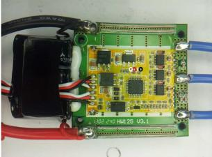
The ESC supports 5S to 12S operation. Switching speed is quite fast. Both low and high side fets are Nfets. Hobbywing Skywalker 12A:
