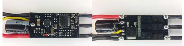
The ESC supports 3S to 6S operation. It supports damped light mode. It does not support low voltage limiting, and it is disabled. Switching speed is quite fast, it has dedicated driver chips. The MCU runs at 48MHz. Both low and high side fets are Nfets. It uses the " XRotor\_20A\_.." code.
