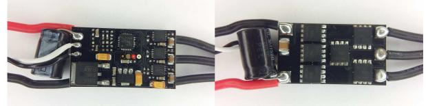
The ESC supports 2S to 6S operation. It supports damped light mode. Switching speed is fast, it has dedicated driver chips. The MCU runs at 48MHz. Both low and high side fets are Nfets.
