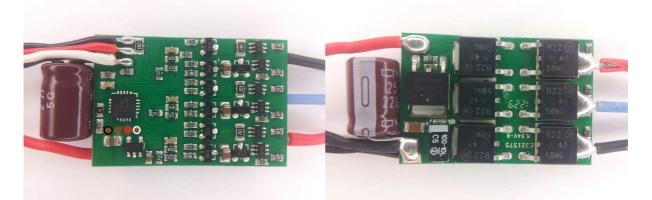
The ESC supports 2S to 4S operation. Switching speed is quite slow. Fet resistances are around 5mohm for low side and high side (typ at 10V). Both low and high side fets are Nfets.
