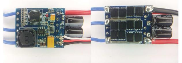
The ESC supports 2S to 6S operation. It supports damped light mode. Switching speed is quite fast. Fet resistances are around 0.75mohm for low side and high side (typ at 10V).
