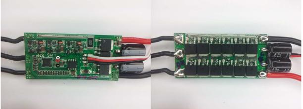
The ESC supports 2S to 3S operation. It supports damped light mode. Switching speed is quite fast. Fet resistances are around 3mohm for low side and high side (max at 10V).
