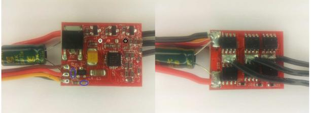
The ESC supports 1S to 3S operation. Switching speed is slow.
