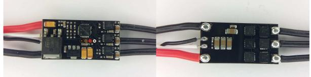
The ESC supports 2S to 4S operation. It supports damped light mode. Switching speed is fast, it has dedicated driver chips. The MCU runs at 48MHz. Both low and high side fets are Nfets.
