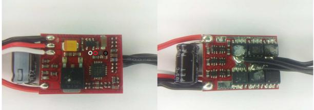
The ESC supports 2S to 4S operation. Switching speed is not fast, ~4.5us (on 2S) for pfet to go off. Also, there is a 2.5us delay in the fet driver that shifts throttle range up, and causes a step in the response from almost full to full throttle. The ESC is the same as the Plush 12A. It uses the same code as the Turnigy Plush 12A.
