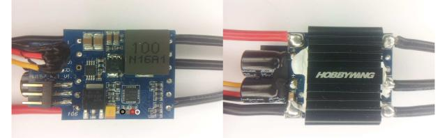
The ESC supports 2S to 6S operation. It supports damped light mode. It supports triple voltage BEC and RPM output. Switching speed is quite fast. The MCU runs at 48MHz. Both low and high side fets are Nfets.
