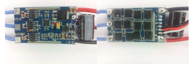
The ESC supports 2S to 6S operation. It supports damped light mode.
