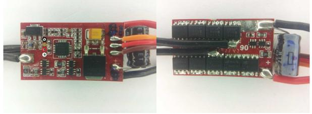
The ESC supports 2S to 3S operation. Switching speed is slow. Fet resistances are around 3mohm for N and 5mohm for P (at 10V).
