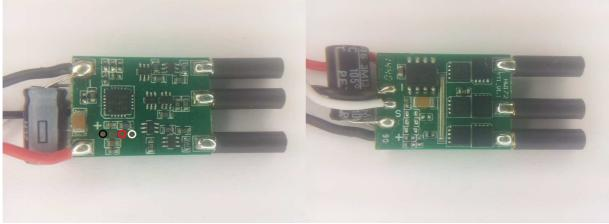
The ESC supports 2S to 3S operation. It supports damped light mode. It does not support low voltage limiting, and it is disabled. Switching speed is somewhat fast. The MCU runs at 48MHz. Low side is Nfets and high side is Pfets.
