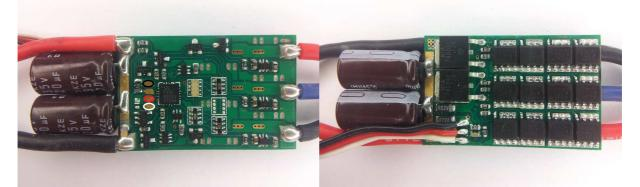
The ESC supports 2S to 4S operation. It supports damped light mode. It supports dual voltage BEC, but beware that the low voltage is below 5V. Switching speed is quite fast.
