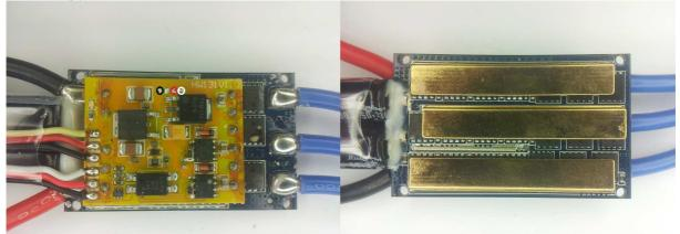
The ESC supports 5S to 12S operation. Switching speed is quite fast. Both low and high side fets are Nfets.
