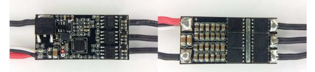
The ESC supports 2S to 6S operation. It supports damped light mode. Switching speed is fast, it has dedicated driver chips. The MCU runs at 48MHz. Both low and high side fets are Nfets.
