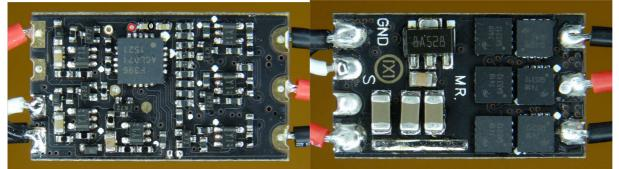
The ESC supports 2S to 4S operation. It supports damped light mode. Switching speed is quite fast. The MCU runs at 48MHz. Both low and high side fets are Nfets.
