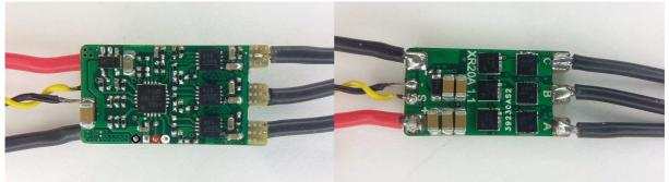
The ESC supports 2S to 4S operation. It supports damped light mode. Switching speed is quite fast. The MCU runs at 48MHz. Both low and high side fets are Nfets. TBS Cube 12A:
