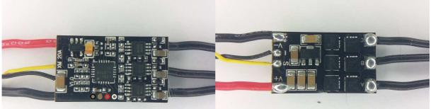
The ESC supports 3S to 4S operation. It supports damped light mode. It does not support low voltage limiting, and it is disabled. Switching speed is fast, it has dedicated driver chips. The MCU runs at 48MHz. Both low and high side fets are Nfets. It uses the "DYS\_XM20A\_.." code. It has also been supplied with the "XRotor\_20A\_.." code, but it will run better with the dedicated code.
