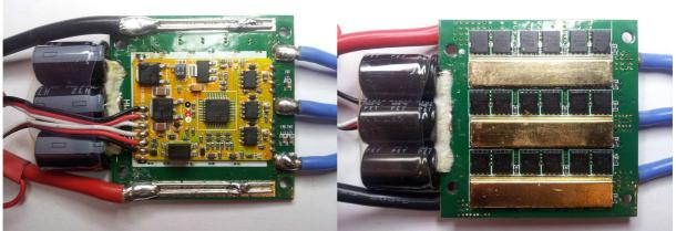
The ESC supports 5S to 12S operation. Switching speed is quite fast. Fet resistances are around 0.8mohm for low side and high side (typ at 10V). Both low and high side fets are Nfets.
