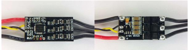
The ESC supports 2S to 3S operation. It supports damped light mode. It does not support low voltage limiting, and it is disabled. Switching speed is somewhat fast. The MCU runs at 48MHz. Low side is Nfets and high side is Pfets. It uses the "XRotor 10A ..." code.
