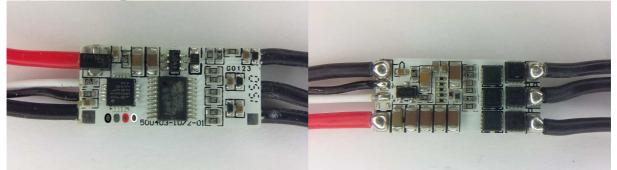
The ESC supports 2S to 4S operation. It supports damped light mode. Switching speed is very fast, it has dedicated driver chips. Both low and high side fets are Nfets.
