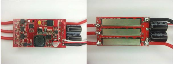
The ESC supports 2S to 6S operation. Switching speed is quite fast. Fet resistances are around 0.7mohm for low side and high side (typ at 10V). Both low and high side fets are Nfets.
