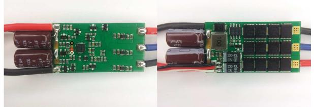
The ESC supports 2S to 4S operation. It supports damped light mode. It supports dual voltage BEC, but beware that the low voltage is below 5V. Switching speed is quite fast.
