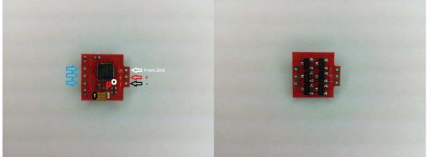
The ESC supports 1S operation only. It supports damped light mode. Switching speed is fast, <0.5us.
