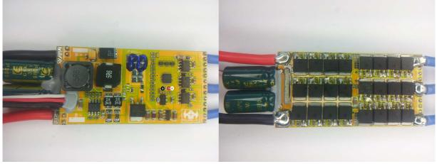
The ESC supports 2S to 6S operation. Switching speed is quite fast. Fet resistances are around 0.65mohm for low side and high side (at 10V).
