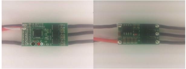
The ESC supports 2S to 4S operation. It supports damped light mode. Switching speed is fast, it has dedicated driver chips. Both low and high side fets are Nfets. FVT Littlebee 20A Pro:
