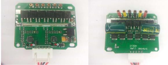
The ESC supports 2S to 6S operation. Switching speed is quite fast.
