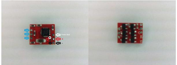
The ESC supports 1S operation only. It supports damped light mode. Switching speed is fast, <0.5us. Fet resistances are approximately 30mohm for N and 60mohm for P.
