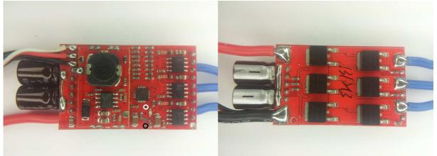
The ESC supports 2S to 4S operation. It supports damped light mode. Switching speed is quite fast. Both low and high side fets are Nfets.
