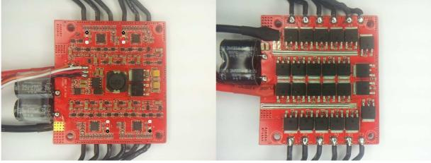
The ESC supports 2S to 6S operation. Switching speed is quite fast. Both low and high side fets are Nfets.
