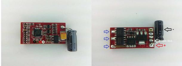
The ESC supports 2S (to 3S) operation. Switching speed is not fast, ~2.5us (on 2S) for pfet to go off. Fet resistances are around 40mohm for N and 60mohm for P (max at 4.5V). Also, there is a 2.5us delay in the fet driver that shifts throttle range up, and causes a step in the response from almost full to full throttle. The ESC is also sold as Hobbywing Flyfun and HiModel Professional.
