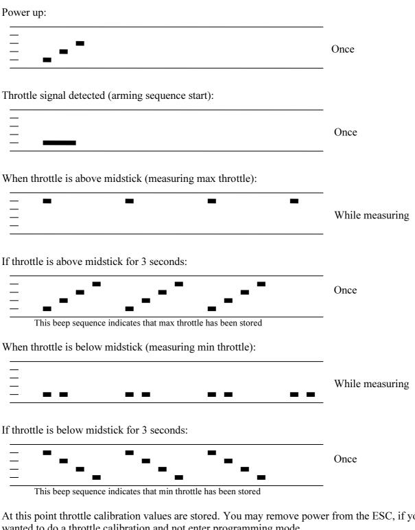
At this point throttle calibration values are stored. You may remove power from the ESC, if you just wanted to do a throttle calibration and not enter programming mode.
