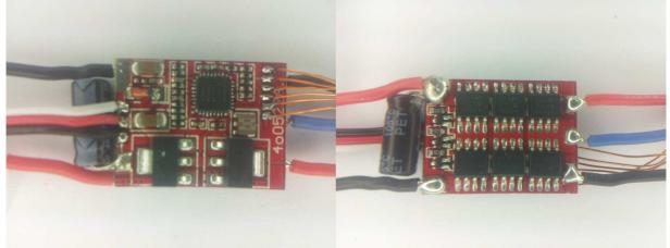
The ESC supports 2S to 3S operation. It supports overtemp protection and bootloader on input plug. Switching speed for high side to turn off is slow. Low side are Nfets and high side are Pfets. It uses the "HK\_UBEC\_10A\_.." code.
