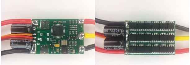
The ESC supports 2S to 4S operation. It does not support bootloader on input plug It does not support overtemp protection. Switching speed for high side to turn off is slow. Low side are Nfets and high side are Pfets. It uses the "Multistar\_30A\_.." code.
