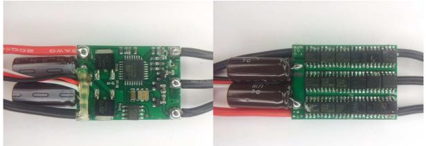
The ESC supports 2S to 3S operation. It supports bootloader on input plug. It does not support overtemp protection. Switching speed for high side to turn off is slow. Low side are Nfets and high side are Pfets. It uses the "SuperSimple\_30A\_.." code.
