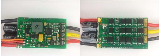
The ESC supports 2S to 6S operation. It supports damped light mode, It does not support bootloader on input plug. It does not support overtemp protection. Switching speed is fast. Both high side and low side are Nfets. It uses the "Multistar\_45A\_.." code.
