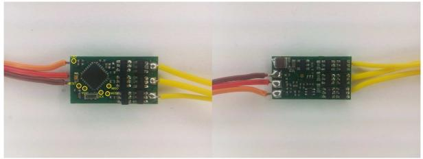
The ESC supports 1S to 2S operation. It supports bootloader on input plug. It does not support overtemp protection. Switching speed for high side to turn off is slow. Low side are Nfets and high side are Pfets. Fuse bytes are (E/H/L): 0xFC/0xDD/0xFF It uses the "YEP\_7A\_.." code. Armattan 12A:
