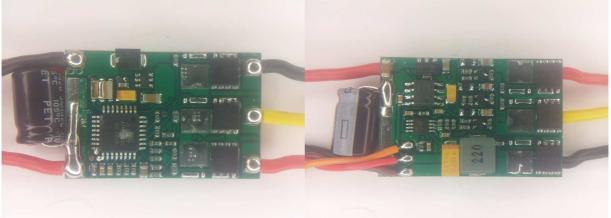
The ESC supports 2S to 6S operation. It supports damped light mode and bootloader on input plug. It does not support overtemp protection. It does not support low voltage limiting. Switching speed is quite fast, although high side is slow to turn on. Both high side and low side are Nfets. It uses the "Multistar\_20Av2\_.." code.
