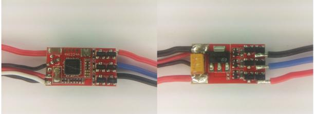
The ESC supports 2S to 3S operation. It supports overtemp protection and bootloader on input plug. Switching speed for high side to turn off is slow. Low side are Nfets and high side are Pfets. It uses the "HK UBEC 6A .." code.
