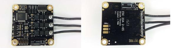
The ESC supports 2S to 4S operation. It supports damped light mode. It supports bootloader on input plug (ICP1).
