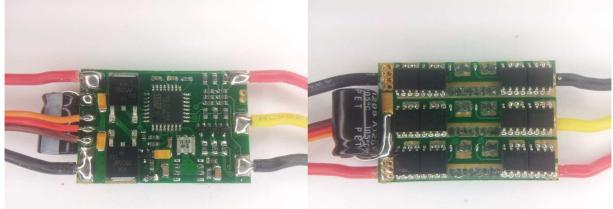
The ESC supports 2S to 3S operation. It does not support bootloader on input plug. It does not support overtemp protection. Switching speed for high side to turn off is slow. Low side are Nfets and high side are Pfets. It uses the "Multistar\_20A\_.." code.
