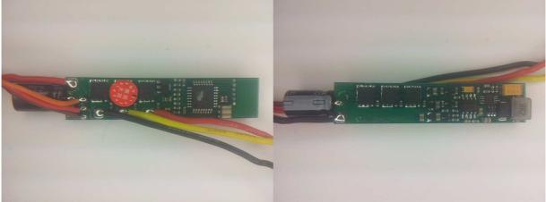
The ESC supports 2S to 6S operation. It supports damped light mode and bootloader on input plug. It does not support overtemp protection. It does not support low voltage limiting. Switching speed is quite fast, although high side is slow to turn on. Both high side and low side are Nfets. It uses the "Multistar\_20Av2\_.." code.
