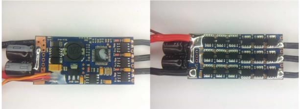
The ESC supports 2S to 6S operation. It supports overtemp protection and bootloader on input plug. Switching speed is quite fast. Both high side and low side are Nfets. It uses the "BlueSeries 40A ..." code.
