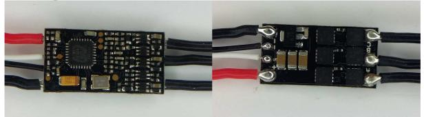
The ESC supports 2S to 4S operation. It supports damped light mode and bootloader on input plug. It does not support overtemp protection. Switching speed is quite fast. Both high side and low side are Nfets. It uses the "ZTW Spider Lite 18Av2 .." code.
