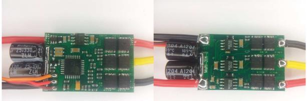
The ESC supports 2S to 6S operation. It supports damped light mode. It does not support bootloader on input plug. It does not support overtemp protection. Switching speed is fast. Both high side and low side are Nfets. It uses the "Sunrise\_HiMulti\_30A\_.." code.
