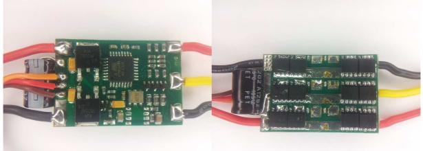
The ESC supports 2S to 3S operation. It does not support bootloader on input plug. It does not support overtemp protection. Switching speed for high side to turn off is slow. Low side are Nfets and high side are Pfets. It uses the "Multistar\_15A\_.." code.
