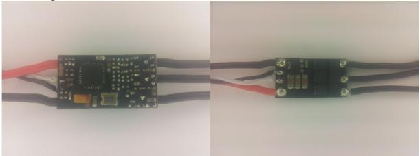
The ESC supports 2S to 4S operation. It supports damped light mode and bootloader on input plug. It does not support overtemp protection. It does not support low voltage limiting. Switching speed is quite fast, although high side is slow to turn on. Both high side and low side are Nfets. It uses the "BlueSeries\_20A\_.." code.
