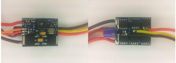
The ESC supports 2S to 3S operation. It supports bootloader on input plug. It does not support overtemp protection. Switching speed for high side to turn off is slow. Low side are Nfets and high side are Pfets. It uses the "Multistar\_10Av2\_.." code.
