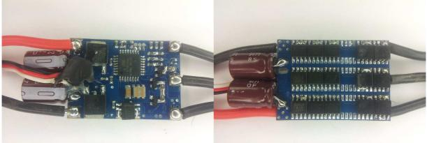
The ESC supports 2S to 3S operation. It supports bootloader on input plug. It does not support overtemp protection. Switching speed for high side to turn off is slow. Low side are Nfets and high side are Pfets. It uses the "SuperSimple\_30A\_.." code.
