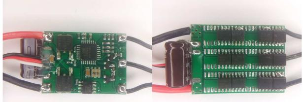
The ESC supports 2S to 3S operation. It supports bootloader on input plug. It does not support overtemp protection. Switching speed for high side to turn off is slow. Low side are Nfets and high side are Pfets. It uses the "SuperSimple 18A ..." code.
