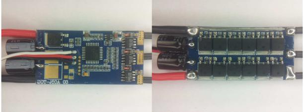
The ESC supports 2S to 6S operation. It supports damped light mode. It supports overtemp protection and bootloader on input plug. Switching speed is fast. Both high side and low side are Nfets. It uses the "RCTimer\_40A\_.." code.
