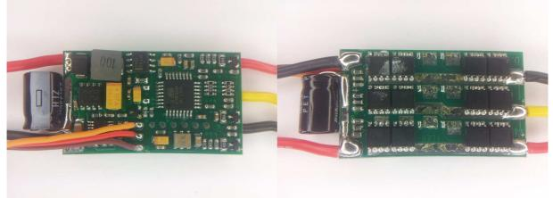
The ESC supports 2S to 4S operation. It does not support bootloader on input plug. It does not support overtemp protection. Switching speed for high side to turn off is slow. Low side are Nfets and high side are Pfets. It uses the "Multistar\_20A\_.." code.
