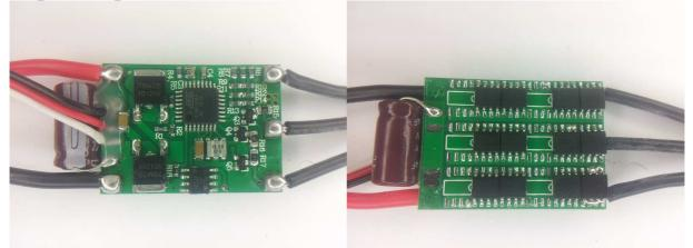
The ESC supports 2S to 3S operation. It supports bootloader on input plug. It does not support overtemp protection. Switching speed for high side to turn off is slow. Low side are Nfets and high side are Pfets. It uses the "SuperSimple\_20A\_.." code.
