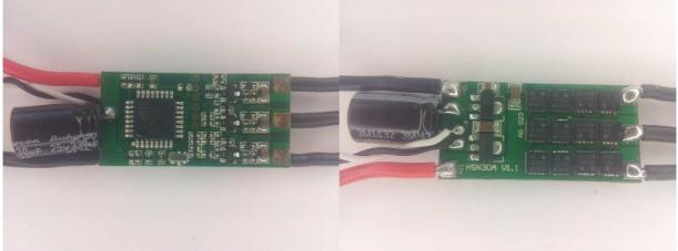
The ESC supports 2S to 6S operation. It supports damped light mode. It supports overtemp protection and bootloader on input plug (ICP1). Since it uses ICP1 as input, it runs smooth also with OneShot125 input signal. Switching speed is quite fast, although high side is slow to turn on. Both high side and low side are Nfets.
