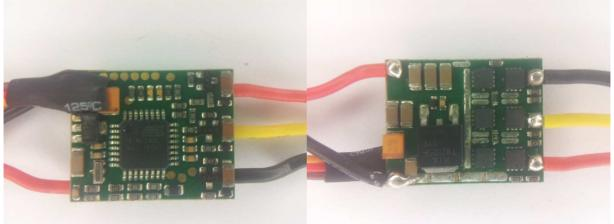
The ESC supports 2S to 4S operation. It supports damped light mode. It supports overtemp protection and bootloader on input plug (ICP1). Since it uses ICP1 as input, it runs smooth also with OneShot125 input signal. Switching speed is quite fast, although high side is slow to turn on. Both high side and low side are Nfets. It uses the "Afro\_12A\_.." code.
