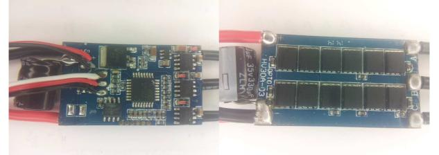
The ESC supports 2S to 6S operation. It supports damped light mode. It supports bootloader on input plug. It does not support overtemp protection. Switching speed is fast. Both high side and low side are Nfets. It uses the "RCTimer 40A ..." code.
