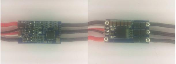
The ESC supports 2S to 4S operation. It supports damped light mode. It supports overtemp protection and bootloader on input plug. Switching speed is quite fast, although high side is slow to turn on. Both high side and low side are Nfets. It uses the "BlueSeries\_20A\_.." code.
