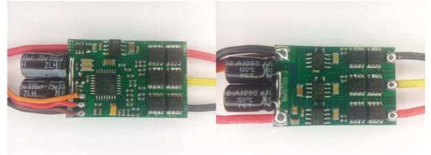
The ESC supports 2S to 6S operation. It supports damped light mode. It does not support bootloader on input plug. It does not support overtemp protection. Switching speed is fast. Both high side and low side are Nfets. It uses the "Sunrise HiMulti 20A ..." code.
