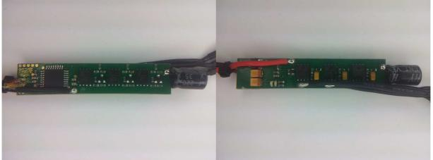
The ESC supports 2S to 4S operation. It supports damped light mode. It supports overtemp protection and bootloader on input plug (ICP1). Since it uses ICP1 as input, it runs smooth also with OneShot125 input signal. Switching speed is quite fast, although high side is slow to turn on. Both high side and low side are Nfets. It uses the "Afro\_20A\_.." code.
