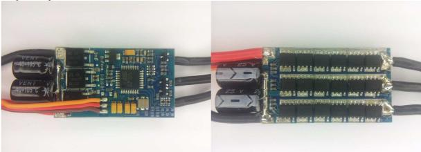
The ESC supports 2S to 3S operation. It supports overtemp protection and bootloader on input plug. Switching speed for high side to turn off is slow. Low side are Nfets and high side are Pfets. At 2S, low voltage limiting does not work reliably. It uses the "Mystery\_30A\_.." code.
