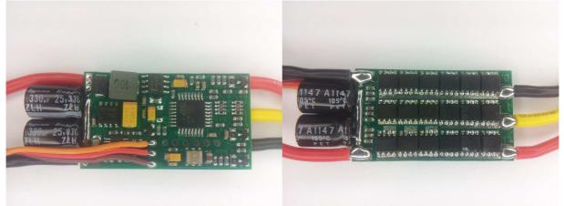
The ESC supports 2S to 4S operation. It does not support bootloader on input plug. It does not support overtemp protection. Switching speed for high side to turn off is slow. Low side are Nfets and high side are Pfets. It uses the "Multistar\_30A\_.." code.
