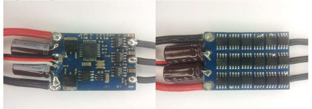
The ESC supports 2S to 3S operation. It supports damped light mode and bootloader on input plug. It does not support overtemp protection. Switching speed is quite fast. Both high side and low side are Nfets. It uses the "SuperSimple\_40A\_.." code.
