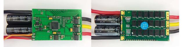
The ESC supports 2S to 10S operation. It supports damped light mode and bootloader on input plug. It does not support overtemp protection. Switching speed is fast. Both high side and low side are Nfets. It uses the "Multistar\_40Av2\_.." code.
