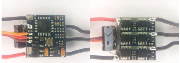
The ESC supports 2S to 3S operation. It supports overtemp protection and bootloader on input plug. Switching speed for high side to turn off is slow. Low side are Nfets and high side are Pfets. At 2S, low voltage limiting does not work reliably. It uses the "Mystery 12A ..." code.
