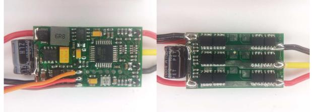
The ESC supports 2S to 4S operation. It does not support bootloader on input plug. It does not support overtemp protection. Switching speed for high side to turn off is slow. Low side are Nfets and high side are Pfets. It uses the "Multistar\_20A\_.." code.
