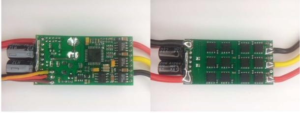
The ESC supports 2S to 6S operation. It supports damped light mode. It does not support bootloader on input plug. It does not support overtemp protection. Switching speed is fast. Both high side and low side are Nfets. It uses the "Sunrise HiMulti 40A ..." code.
