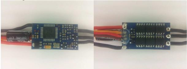
The ESC supports 2S to 4S operation. It supports damped light mode and bootloader on input plug. It does not support overtemp protection. It does not support low voltage limiting. Switching speed is quite fast, although high side is slow to turn on. Both high side and low side are Nfets.
