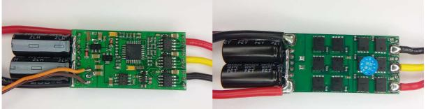
The ESC supports 2S to 8S operation. It supports damped light mode and bootloader on input plug. It does not support overtemp protection. Switching speed is fast. Both high side and low side are Nfets. It uses the "Multistar\_40Av2\_.." code.
