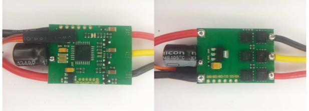
The ESC supports 2S to 4S operation. It supports damped light mode. It supports overtemp protection and bootloader on input plug (ICP1). Since it uses ICP1 as input, it runs smooth also with OneShot125 input signal. Switching speed is quite fast, although high side is slow to turn on. Both high side and low side are Nfets. It uses the "Afro\_30A\_.." code.
