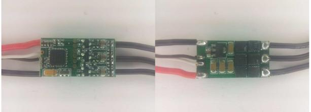
The ESC supports 2S to 4S operation. It supports damped light mode. It supports overtemp protection and bootloader on input plug (ICP1). Since it uses ICP1 as input, it runs smooth also with OneShot125 input signal. Switching speed is quite fast, although high side is slow to turn on. Both high side and low side are Nfets.
