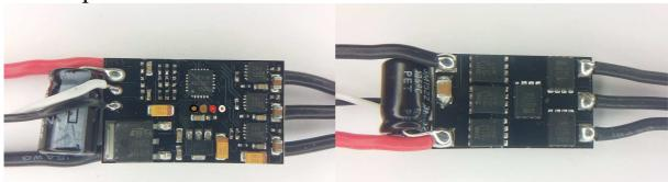
The ESC supports 2S to 6S operation. It supports damped light mode. Switching speed is fast, it has dedicated driver chips. The MCU runs at 48MHz.
