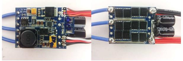
The ESC supports 2S to 6S operation. It supports damped light mode. It supports dual voltage BEC.
