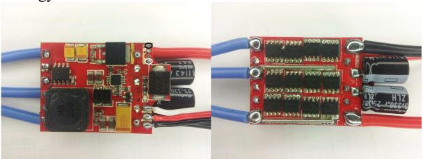
The ESC supports 2S to 6S operation. It supports damped light mode.
