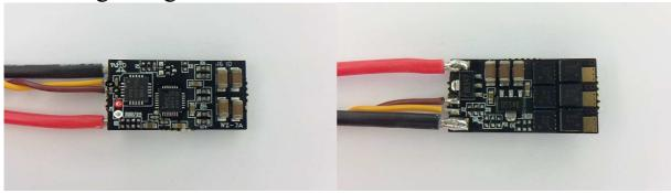
The ESC supports 2S to 4S operation. It supports damped light mode. Switching speed is fast, it has dedicated driver chips with automatic deadtime. The MCU runs at 48MHz.
