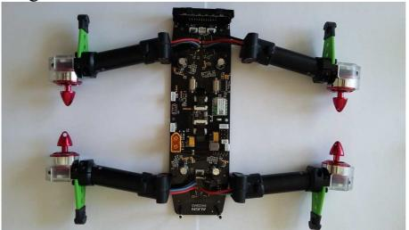
The ESC supports 3S to 4S operation. It supports damped light mode. The ESCs are integrated in the bottom plate board. Switching speed is quite fast.
