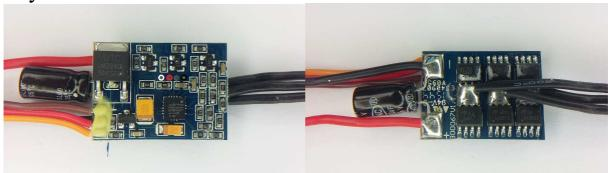
The ESC supports 2S to 3S operation. Switching speed is not fast, pfets are slow to go off. It uses the "XP\_12A\_.." code.
