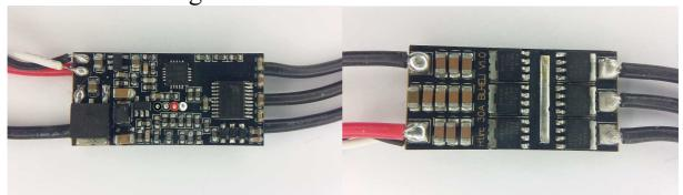
The ESC supports 2S to 6S operation. It supports damped light mode. Switching speed is fast, it has dedicated driver chips. The MCU runs at 48MHz.
