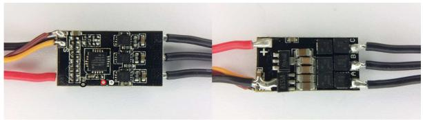
The ESC supports 3S to 4S operation. It supports damped light mode. Switching speed is fast, it has dedicated driver chips. Both low and high side fets are Nfets. It uses the "Emax Nano 20A ..." code.
