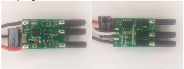
The ESC supports 2S to 3S operation. It supports damped light mode. It does not support low voltage limiting, and it is disabled. Switching speed is somewhat fast.
