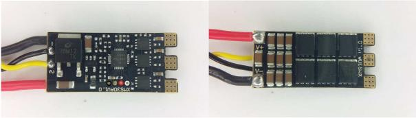
The ESC supports 3S to 6S operation. It supports damped light mode. It does not support low voltage limiting, and it is disabled. Switching speed is fast, it has dedicated driver chips. The MCU runs at 48MHz. Both low and high side fets are Nfets.
