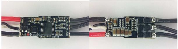
The ESC supports 2S to 4S operation. It supports damped light mode. Switching speed is fast, it has dedicated driver chips. Both low and high side fets are Nfets.
