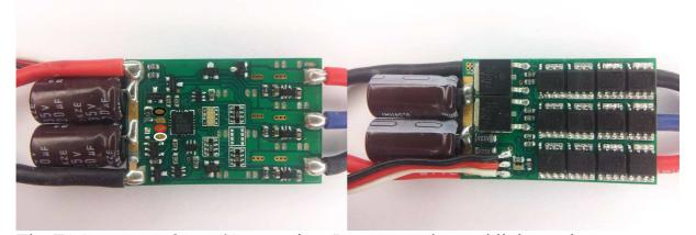
The ESC supports 2S to 4S operation. It supports damped light mode. Switching speed is quite fast.
