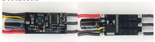
The ESC supports 3S to 6S operation. It supports damped light mode. It does not support low voltage limiting, and it is disabled. Switching speed is quite fast, it has dedicated driver chips. The MCU runs at 48MHz. Both low and high side fets are Nfets. It uses the "XRotor 20A .." code.
