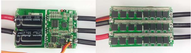
The ESC supports up to 12S operation. It supports damped light mode. Switching speed is fast, it has dedicated driver chips. Both low and high side fets are Nfets.
