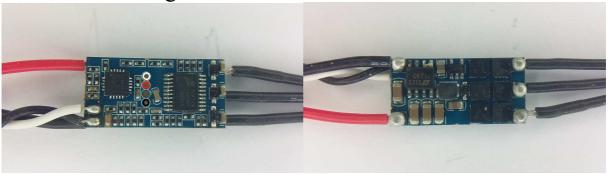
The ESC supports 2S to 4S operation. It supports damped light mode. Switching speed is fast, it has dedicated driver chips. Both low and high side fets are Nfets.
