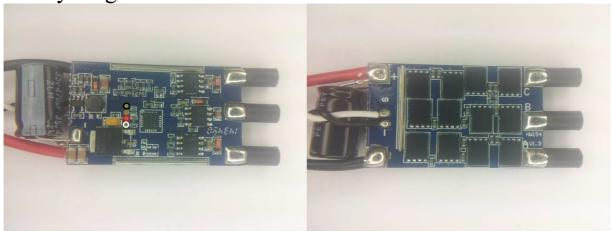
The ESC supports 2S to 6S operation. It supports damped light mode. It does not support low voltage limiting, and it is disabled. Switching speed is fast.
