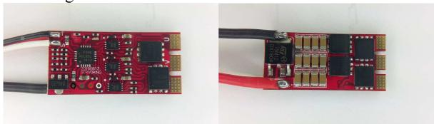
The ESC supports 3S to 5S operation. It supports damped light mode. Switching speed is fast, it has dedicated driver chips. The MCU runs at 48MHz.
