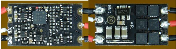
The ESC supports 2S to 4S operation. It supports damped light mode. Switching speed is quite fast.
