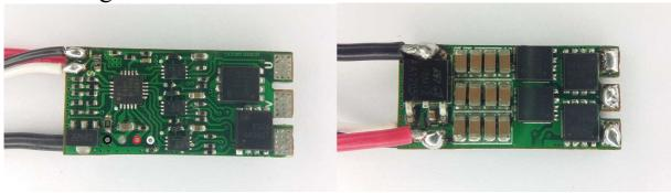
The ESC supports 3S to 5S operation. It supports damped light mode. Switching speed is fast, it has dedicated driver chips. Both low and high side fets are Nfets.
