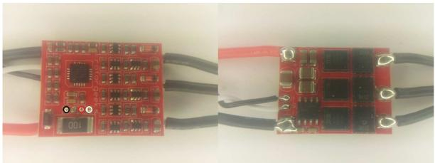
The ESC supports 2S to 4S operation. It supports damped light mode. Switching speed is fast.
