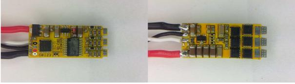
The ESC supports 2S to 4S operation. It supports damped light mode. Switching speed is fast, it has dedicated driver chips.
