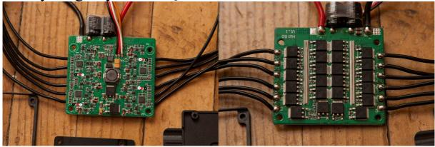
The ESC supports 2S to 3S operation. It supports damped light mode. Switching speed is quite fast.
