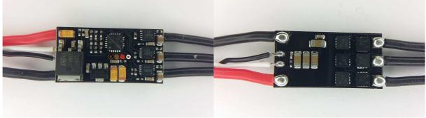
The ESC supports 2S to 4S operation. It supports damped light mode. Switching speed is fast, it has dedicated driver chips. The MCU runs at 48MHz.
