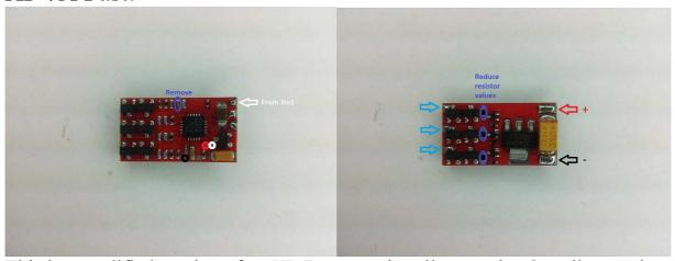
This is a modified version of an XP 7A esc, primarily targeting 2S tail operation. The ESC supports 1S to 2S operation. It supports damped light mode.
