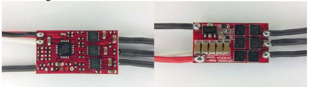
The ESC supports 2S to 4S operation. It supports damped light mode. Switching speed is fast, it has dedicated driver chips. Both low and high side fets are Nfets. It uses the "FVT LITTLEBEE 20A.." code.
