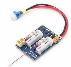
The ESC supports 1S to 2S operation. Switching speed is not fast.
