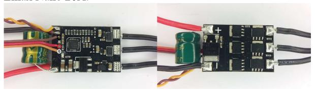
The ESC supports 3S to 4S operation. It supports damped light mode. Switching speed is fast, it has dedicated driver chips. Both low and high side fets are Nfets.
