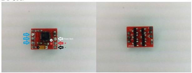
The ESC supports 1S operation only. It supports damped light mode. Switching speed is fast, <0.5us.
