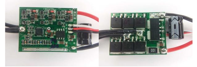
The ESC supports 2S to 3S operation. It supports damped light mode. Switching speed is quite fast.
