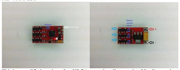
This is a modified version of an XP 7A esc, primarily targeting 2S tail operation. The ESC supports 1S to 2S operation. It supports damped light mode. Switching speed is modified to be faster, ~1.6us (on 2S) for pfet to go off, thereby enabling damped mode operation.
