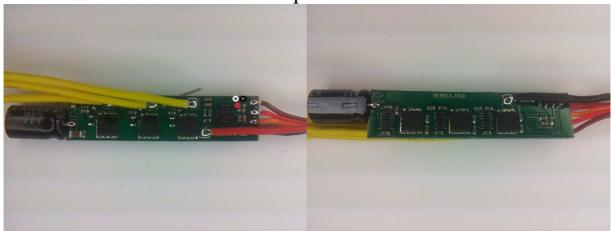
The ESC supports 2S to 4S operation. It supports damped light mode. Switching speed is quite fast.
