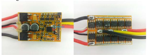
The ESC supports 2S to 3S operation. It supports damped light mode. Switching speed is quite fast.
