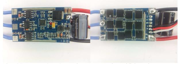
The ESC supports 2S to 6S operation. It supports damped light mode. Switching speed is quite fast.
