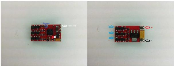
The ESC supports 1S to 2S operation. Switching speed is not fast, ~5us (on 2S) for pfet to go off. Fet resistances are around 12mohm for N and 30mohm for P (typ at 2.5V). The circled capacitor in the image above should be removed for high frequency input signals (pwm > 1kHz, e.g. mCPX v1).
