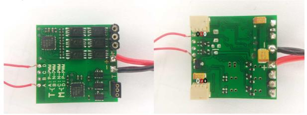
The ESC supports 1S operation, and has both a 10A main and a 3A tail ESC. Switching speed of main is not fast, ~5us (on 2S) for pfet to go off. Switching speed of tail is fast, <0.5us.
