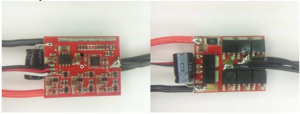
The ESC supports 2S to 4S operation. Switching speed is quite fast. Both low and high side fets are Nfets.
