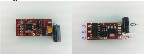
The ESC supports 2S (to 3S) operation. Switching speed is not fast, ~2.5us (on 2S) for pfet to go off. Fet resistances are around 40mohm for N and 60mohm for P (max at 4.5V). Also, there is a 2.5us delay in the fet driver that shifts throttle range up, and causes a step in the response from almost full to full throttle.
