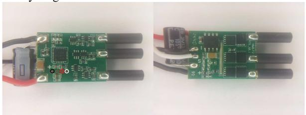
The ESC supports 2S to 3S operation. It supports damped light mode. It does not support low voltage limiting, and it is disabled.
