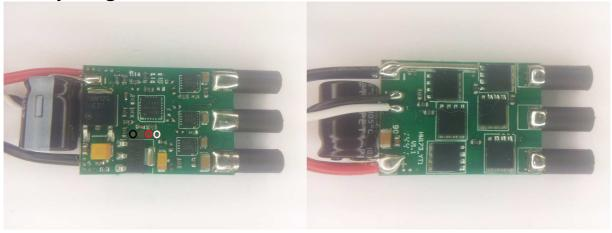
The ESC supports 3S to 4S operation. It supports damped light mode.
