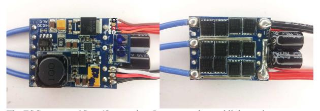
The ESC supports 2S to 6S operation. It supports damped light mode. It supports dual voltage BEC.
