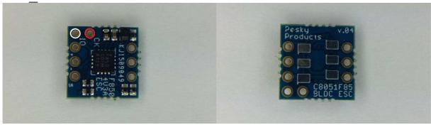
The ESC supports 1S operation only. It supports damped light mode. Switching speed is fast, <0.5us.
