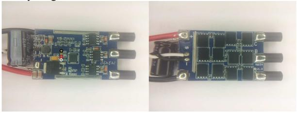
The ESC supports 2S to 6S operation. It supports damped light mode.
