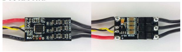
The ESC supports 2S to 3S operation. It supports damped light mode.
