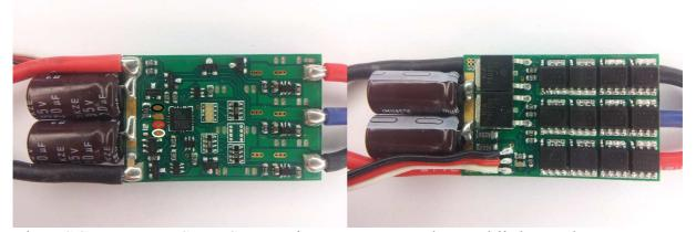
The ESC supports 2S to 4S operation. It supports damped light mode. It supports dual voltage BEC, but beware that the low voltage is below 5V. Switching speed is quite fast.
