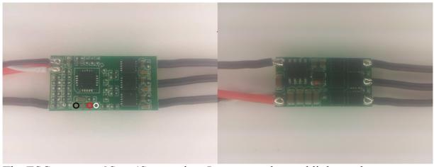
The ESC supports 2S to 4S operation. It supports damped light mode. Switching speed is fast, it has dedicated driver chips. Both low and high side fets are Nfets.
