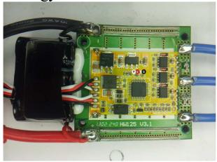
The ESC supports 5S to 12S operation. Switching speed is quite fast. Both low and high side fets are Nfets.
