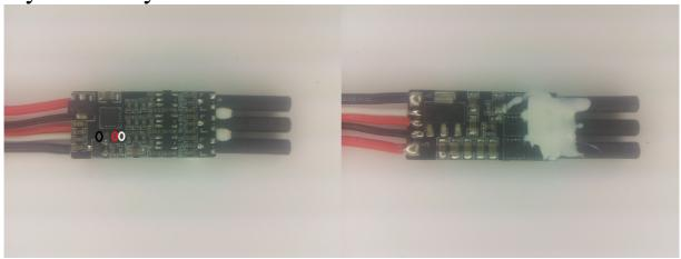
The ESC supports 2S to 4S operation. Switching speed is not fast, high side is slow to turn on. Low side is Nfets and high side is Pfets.
