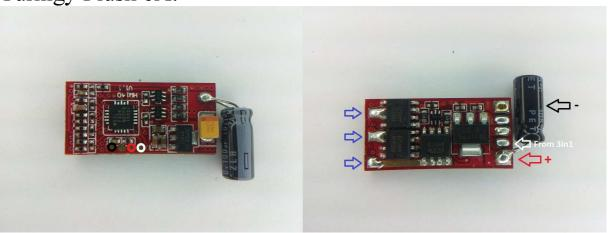
The ESC supports 2S (to 3S) operation. Switching speed is not fast, ~2.5us (on 2S) for pfet to go off. Fet resistances are around 40mohm for N and 60mohm for P (max at 4.5V). Also, there is a 2.5us delay in the fet driver that shifts throttle range up, and causes a step in the response from almost full to full throttle.
