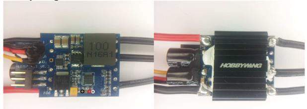
The ESC supports 2S to 6S operation. It supports damped light mode.
