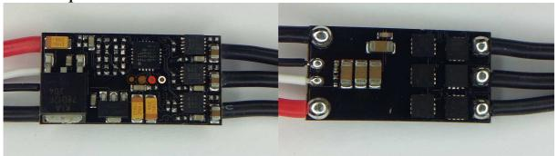
The ESC supports 2S to 4S operation. It supports damped light mode. Switching speed is very fast, it has dedicated driver chips. Both low and high side fets are Nfets.
