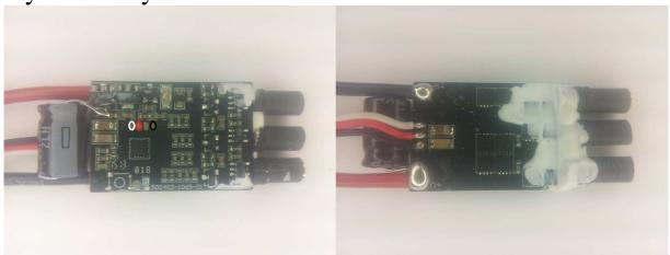
The ESC supports 2S to 6S operation. It supports damped light mode. Switching speed is quite fast, although high side is slow to turn on. Both low and high side fets are Nfets.
