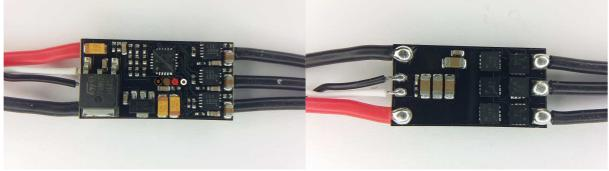
The ESC supports 2S to 4S operation. It supports damped light mode. Switching speed is fast, it has dedicated driver chips. The MCU runs at 48MHz.
