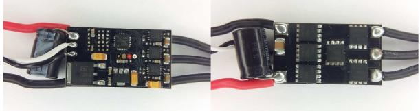
The ESC supports 2S to 6S operation. It supports damped light mode. Switching speed is fast, it has dedicated driver chips. The MCU runs at 48MHz.
