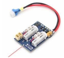
The ESC supports 1S to 2S operation. Switching speed is not fast.
