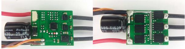
The ESC supports 2S to 4S operation. It supports damped light mode. It does not support low voltage limiting, and it is disabled. Switching speed is fast, it has dedicated driver chips. The MCU runs at 48MHz. Both low and high side fets are Nfets.
