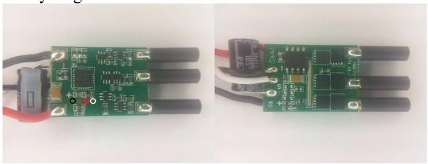
The ESC supports 2S to 3S operation. It supports damped light mode. It does not support low voltage limiting, and it is disabled.
