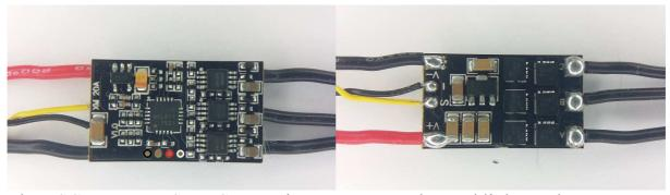
The ESC supports 3S to 4S operation. It supports damped light mode.
