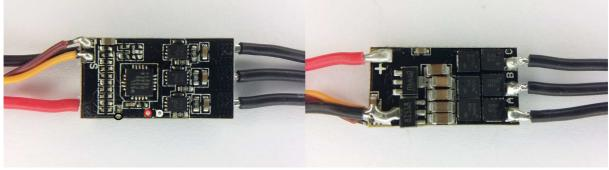
The ESC supports 3S to 4S operation. It supports damped light mode. Switching speed is fast, it has dedicated driver chips. Both low and high side fets are Nfets.
