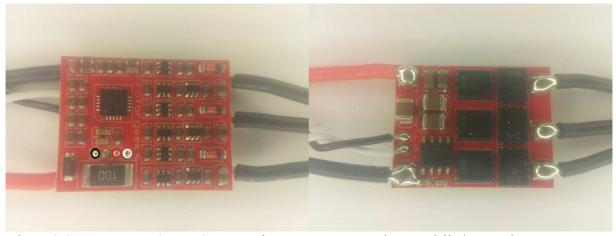
The ESC supports 2S to 4S operation. It supports damped light mode. Switching speed is fast.
