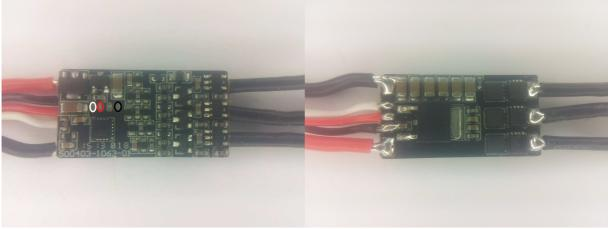
The ESC supports 2S to 4S operation. It supports damped light mode. Switching speed is quite fast, although high side is slow to turn on. Both low and high side fets are Nfets.
