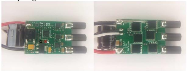
The ESC supports 3S to 4S operation. It supports damped light mode. It does not support low voltage limiting, and it is disabled. Switching speed is somewhat fast.
