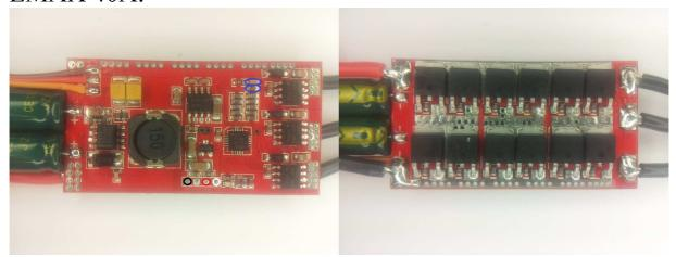
The ESC supports 2S to 6S operation. It supports damped light mode. Switching speed is fast.
