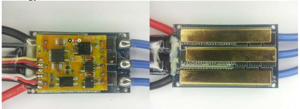
The ESC supports 5S to 12S operation. Switching speed is quite fast. Both low and high side fets are Nfets.
