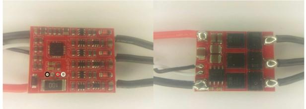
The ESC supports 2S to 4S operation. It supports damped light mode. Switching speed is fast.
