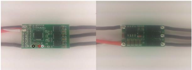
The ESC supports 2S to 4S operation. It supports damped light mode. Switching speed is fast, it has dedicated driver chips. Both low and high side fets are Nfets.
