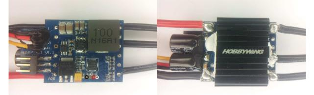
The ESC supports 2S to 6S operation. It supports damped light mode. It supports triple voltage BEC and RPM output. Switching speed is quite fast. The MCU runs at 48MHz. Both low and high side fets are Nfets.
