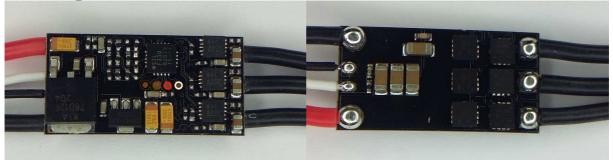
The ESC supports 2S to 4S operation. It supports damped light mode. Switching speed is very fast, it has dedicated driver chips. Both low and high side fets are Nfets.
