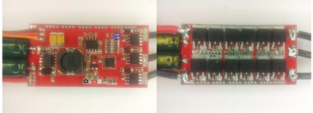
The ESC supports 2S to 6S operation. It supports damped light mode. Switching speed is fast.
