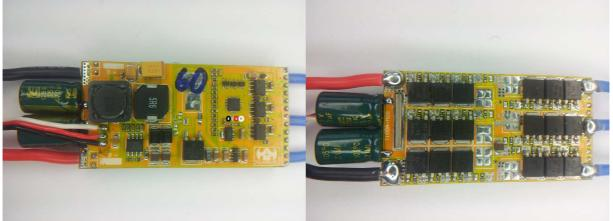
The ESC supports 2S to 6S operation. Switching speed is quite fast. Fet resistances are around 1.1mohm for low side and high side (at 10V). Both low and high side fets are Nfets.
