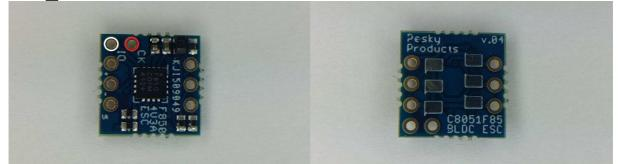
The ESC supports 1S operation only. It supports damped light mode. Switching speed is fast, <0.5us.
