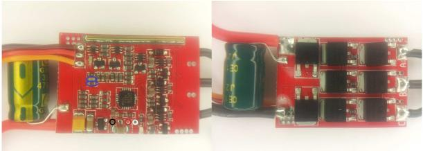
The ESC supports 2S to 3S operation. It supports damped light mode.
