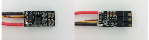
The ESC supports 2S to 4S operation. It supports damped light mode. Switching speed is fast, it has dedicated driver chips with automatic deadtime. The MCU runs at 48MHz.
