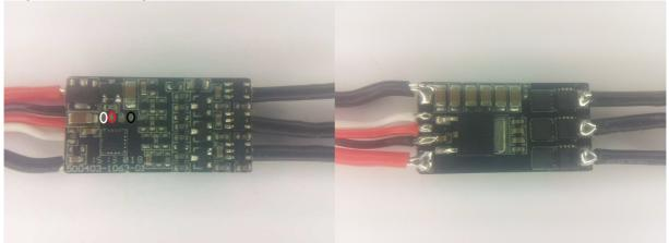
The ESC supports 2S to 4S operation. It supports damped light mode. Switching speed is quite fast, although high side is slow to turn on.
