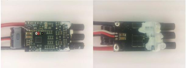
The ESC supports 2S to 6S operation. It supports damped light mode. Switching speed is quite fast, although high side is slow to turn on. Both low and high side fets are Nfets.
