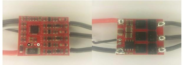
The ESC supports 2S to 4S operation. It supports damped light mode. Switching speed is fast. The MCU runs at 48MHz. Both low and high side fets are Nfets.
