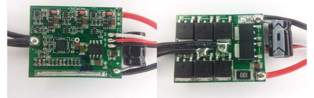
The ESC supports 2S to 3S operation. It supports damped light mode. Switching speed is quite fast.
