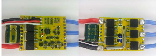
The ESC supports 2S to 4S operation. Switching speed is slow. Fet resistances are around 3.5mohm for low side and high side (at 10V). Both low and high side fets are Nfets.
