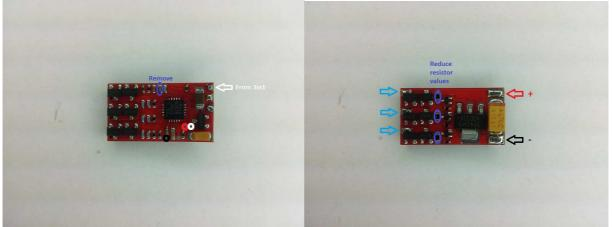
This is a modified version of an XP 7A esc, primarily targeting 2S tail operation. The ESC supports 1S to 2S operation. It supports damped light mode. Switching speed is modified to be faster, ~1.6us (on 2S) for pfet to go off, thereby enabling damped mode operation.
