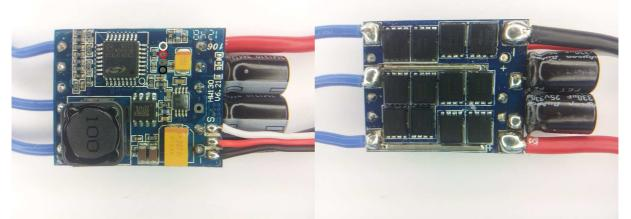
The ESC supports 2S to 6S operation. It supports damped light mode. Switching speed is quite fast. Fet resistances are around 0.75mohm for low side and high side (typ at 10V). Both low and high side fets are Nfets. This ESC uses the same code as the Plush 40A ESC.
