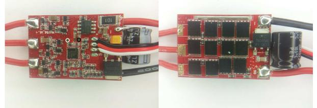
The ESC supports 2S to 4S operation. It supports damped light mode. Switching speed is quite fast.
