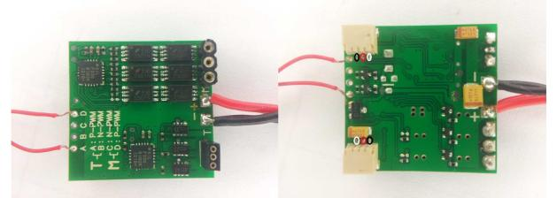
The ESC supports 1S operation, and has both a 10A main and a 3A tail ESC. Switching speed of main is not fast, ~5us (on 2S) for pfet to go off. Switching speed of tail is fast, <0.5us.
