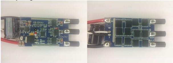
The ESC supports 2S to 6S operation. It supports damped light mode. It does not support low voltage limiting, and it is disabled. Switching speed is fast. The MCU runs at 48MHz. Both low and high side fets are Nfets.
