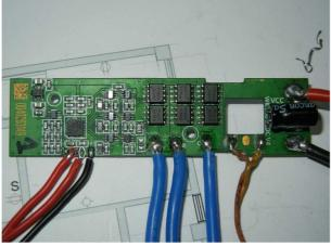
The ESC supports 3S operation. Switching speed is not fast, several us for pfet to go off. This ESC uses the same code as the Turnigy Plush 18A ESC.
