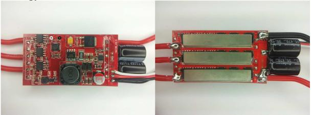
The ESC supports 2S to 6S operation. Switching speed is quite fast. Fet resistances are around 0.7mohm for low side and high side (typ at 10V). Both low and high side fets are Nfets. The ESC is also sold as Hobbywing Flyfun and HiModel Professional.
