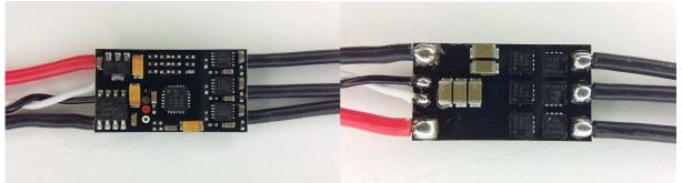
The ESC supports 2S to 4S operation. It supports damped light mode. Switching speed is fast, it has dedicated driver chips. The MCU runs at 48MHz. Both low and high side fets are Nfets.
