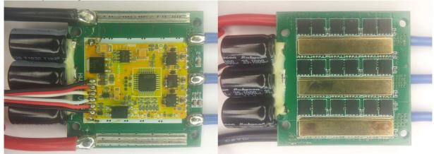
The ESC supports 2S to 6S operation. It supports damped light mode. Switching speed is quite fast. Both low and high side fets are Nfets.
