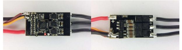
The ESC supports 3S to 4S operation. It supports damped light mode. Switching speed is fast, it has dedicated driver chips. Both low and high side fets are Nfets. It uses the "Emax\_Nano\_20A\_.." code.
