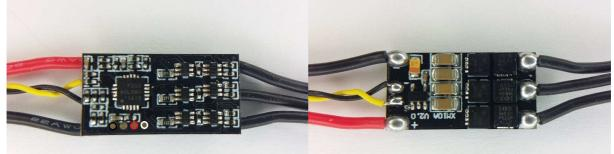
The ESC supports 2S to 3S operation. It supports damped light mode. It does not support low voltage limiting, and it is disabled. Switching speed is somewhat fast. The MCU runs at 48MHz. Low side is Nfets and high side is Pfets. It uses the "XRotor\_10A\_.." code.
