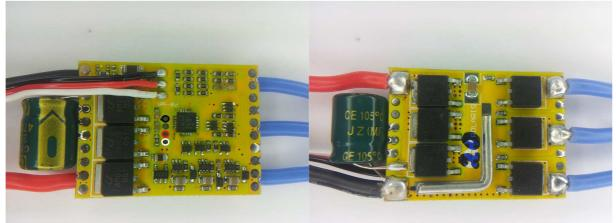
The ESC supports 2S to 4S operation. Switching speed is slow.
