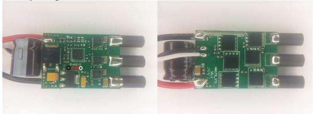
The ESC supports 3S to 4S operation. It supports damped light mode. It does not support low voltage limiting, and it is disabled. Switching speed is somewhat fast. The MCU runs at 48MHz. Both low and high side fets are Nfets.
