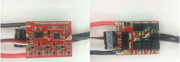
The ESC supports 2S to 4S operation. Switching speed is quite fast. Both low and high side fets are Nfets.
