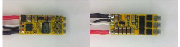
The ESC supports 2S to 4S operation. It supports damped light mode. Switching speed is fast, it has dedicated driver chips. The MCU runs at 48MHz. Both low and high side fets are Nfets.
