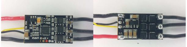
The ESC supports 3S to 4S operation. It supports damped light mode. It does not support low voltage limiting, and it is disabled.
