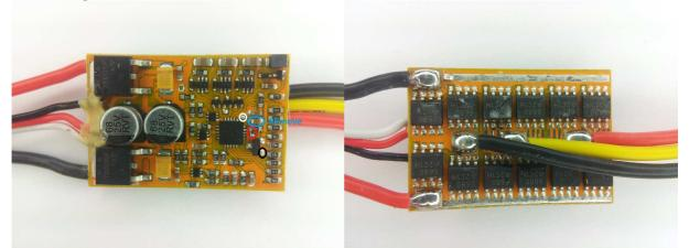
The ESC supports 2S to 3S operation. It supports damped light mode.
