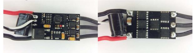
The ESC supports 2S to 6S operation. It supports damped light mode. Switching speed is fast, it has dedicated driver chips. The MCU runs at 48MHz. Both low and high side fets are Nfets.
