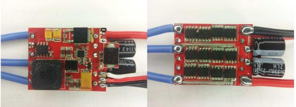
The ESC supports 2S to 6S operation. It supports damped light mode. It supports dual voltage BEC.
