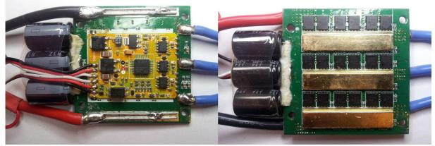
The ESC supports 5S to 12S operation. Switching speed is quite fast. Fet resistances are around 0.8mohm for low side and high side (typ at 10V). Both low and high side fets are Nfets.
