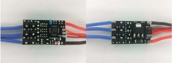
The ESC supports 2S operation. Switching speed is not fast, ~5us (on 2S) for pfet to go off. Fet resistances are around 12mohm for N and 30mohm for P (typ at 2.5V). The circled capacitor in the image above should be removed for high frequency input signals (pwm > 1kHz, e.g. mCPX v1). The ESC is also sold as RCX 6A.
