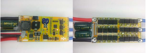
The ESC supports 2S to 6S operation. Switching speed is quite fast. Fet resistances are around 0.65mohm for low side and high side (at 10V). Both low and high side fets are Nfets.
