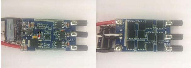
The ESC supports 2S to 6S operation. It supports damped light mode. Switching speed is fast. The MCU runs at 50MHz. Both low and high side fets are Nfets.
