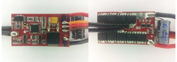
The ESC supports 2S to 3S operation. Switching speed is slow. Fet resistances are around 3mohm for N and 5mohm for P (at 10V).
