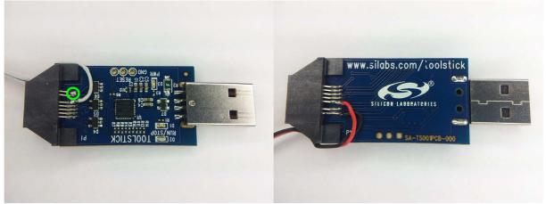
The green circle in the above image indicates where two pins on the connector shall be shorted.
