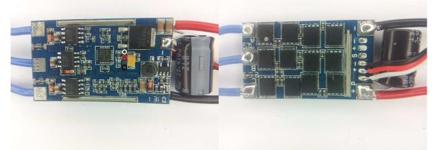
The ESC supports 2S to 6S operation. It supports damped light mode. Switching speed is quite fast.
