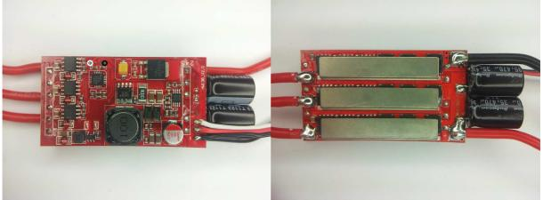
The ESC supports 2S to 6S operation. Switching speed is quite fast.
