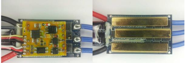
The ESC supports 5S to 12S operation. Switching speed is quite fast. Both low and high side fets are Nfets.
