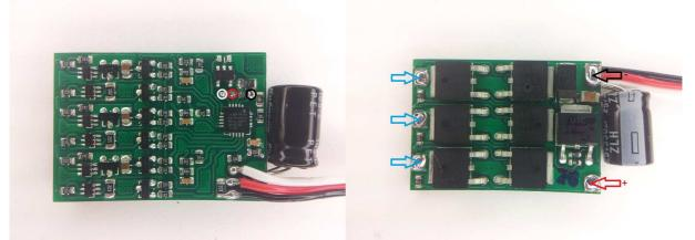
The ESC supports 2S to 4S operation. Switching speed is quite slow. Fet resistances are around 5mohm for low side and high side (typ at 10V). Both low and high side fets are Nfets.
