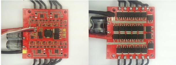
The ESC supports 2S to 6S operation. Switching speed is quite fast. Both low and high side fets are Nfets.
