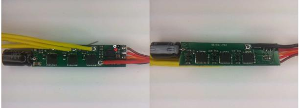
The ESC supports 2S to 4S operation. It supports damped light mode. Switching speed is quite fast. Both low and high side fets are Nfets. This ESC is sold with the "Hobbywing Skywalker 20A" code.
