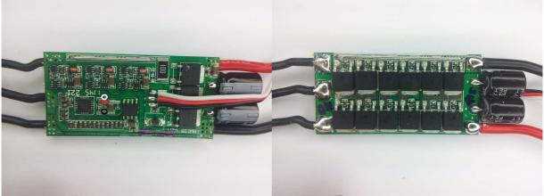
The ESC supports 2S to 3S operation. It supports damped light mode. Switching speed is quite fast.
