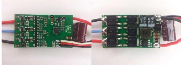
The ESC supports 2S to 4S operation. Switching speed is quite slow. Fet resistances are around 5mohm for low side and high side (typ at 10V). Both low and high side fets are Nfets. The ESC has a switch mode BEC.
