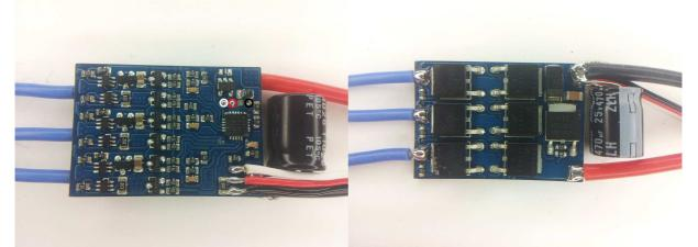
The ESC supports 2S to 4S operation. Switching speed is quite slow. Fet resistances are around 4mohm for low side and high side (max at 10V). Both low and high side fets are Nfets.
