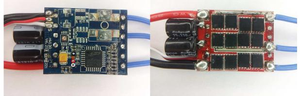
The ESC supports 2S to 6S operation. It supports damped light mode. Switching speed is quite fast.
