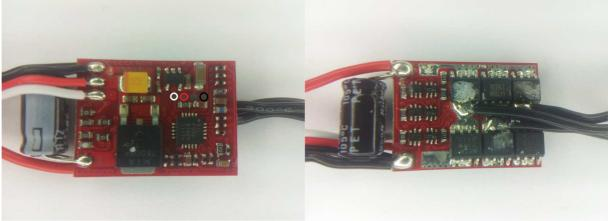
The ESC supports 2S to 4S operation. Switching speed is not fast, ~4.5us (on 2S) for pfet to go off. Also, there is a 2.5us delay in the fet driver that shifts throttle range up, and causes a step in the response from almost full to full throttle. The ESC is the same as the Plush 12A. It uses the same code as the Turnigy Plush 12A.
