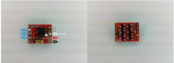
The ESC supports 1S operation only. It supports damped light mode. Switching speed is fast, <0.5us. Fet resistances are approximately 40mohm for N and 90mohm for P.
