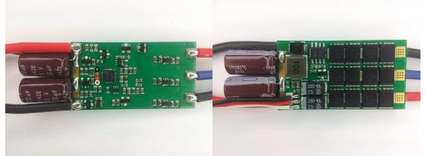
The ESC supports 2S to 4S operation. It supports damped light mode. It supports dual voltage BEC, but beware that the low voltage is below 5V. Switching speed is quite fast.
