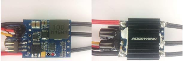
The ESC supports 2S to 6S operation. It supports damped light mode. It supports triple voltage BEC and RPM output. Switching speed is quite fast. The MCU runs at 50MHz. Both low and high side fets are Nfets.
