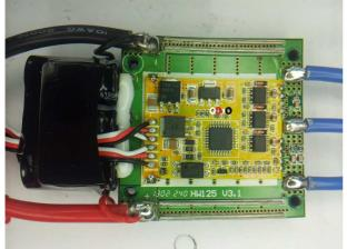
The ESC supports 5S to 12S operation. Switching speed is quite fast. Both low and high side fets are Nfets.
