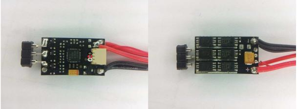
The ESC supports 1S operation. Switching speed is not fast, ~5us (on 2S) for pfet to go off. Fet resistances are around 10mohm for N and 10mohm for P (typ at 2.5V). The ESC has a dedicated connector for programming. It is sold under many brand names, Oversky, Hawk, Xtreme, Airbase and probably more.
