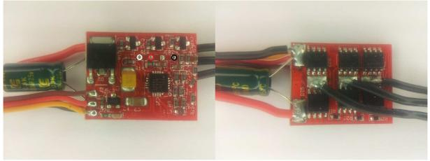
The ESC supports 1S to 3S operation. Switching speed is slow. Low side is Nfets and high side is Pfets. It uses the "XP\_12A\_.." code.
