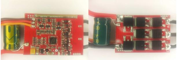
The ESC supports 2S to 3S operation. It supports damped light mode. Switching speed is quite fast. Both low and high side fets are Nfets.
