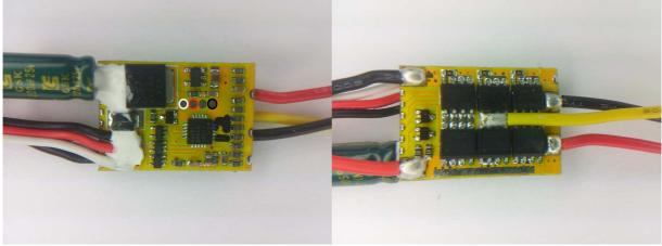
The ESC supports 2S to 3S operation. Switching speed is slow. Fet resistances are around 3mohm for N and 10mohm for P (at 10V).
