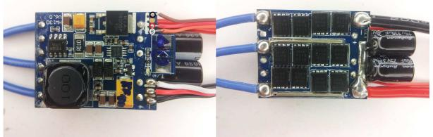
The ESC supports 2S to 6S operation. It supports damped light mode. It supports dual voltage BEC.
