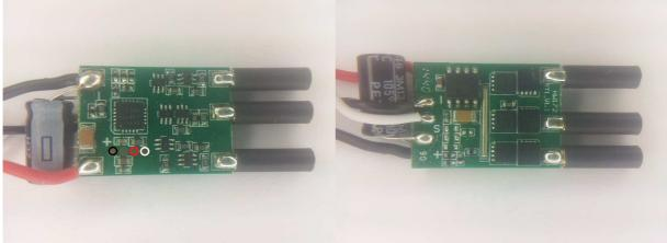
The ESC supports 2S to 3S operation. It supports damped light mode. Switching speed is somewhat fast. The MCU runs at 50MHz. Low side is Nfets and high side is Pfets.
