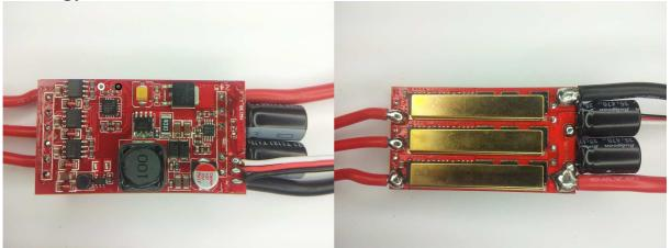
The ESC supports 2S to 6S operation. Switching speed is quite fast. Fet resistances are around 0.5mohm for low side and high side (typ at 10V). Both low and high side fets are Nfets.
