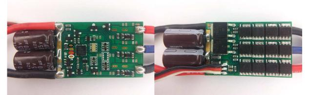
The ESC supports 2S to 4S operation. It supports damped light mode. It supports dual voltage BEC, but beware that the low voltage is below 5V. Switching speed is quite fast.
