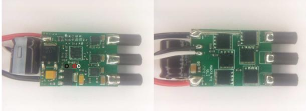
The ESC supports 3S to 4S operation. It supports damped light mode. Switching speed is somewhat fast. The MCU runs at 50MHz. Both low and high side fets are Nfets.
