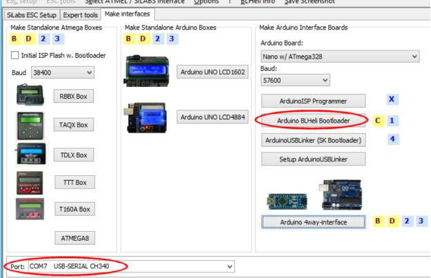
Note that COM7 shown here is just an example. The actual COM port assigned will vary. The appropriate baud rate will change by selection of the Arduino board and is determined by the installed Arduino bootloader. In the shown case 57600 baud is set for the Nano board.
