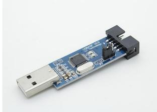
The most convenient adapter to go with the above socket tool, is the USBasp.
