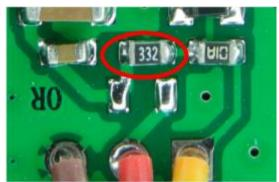
Without modifications this stick can be used with Atmel BLHeli bootloader. In order to use it with SiLabs BLHeli bootloader, it is necessary to change the red circled 3.3Kohm resistor ("332") with a 27 to 47Kohm resistor.
